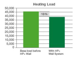
A typical builder using R-19 cavity insulation in 2x6 framing has an effective R-value of 11.8. The HP+ System with continuous insulation, closed cell spray foam and 2x4 advanced framing boosts the effective R to 15.3.
